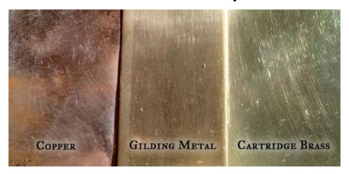
Copper and copper alloys have a wide range of colours. Modern "common brass" (Cu 63% Zn 37% Mix) has a colour that is distinctive as modern brass due to it's zinc content being over 30%.
